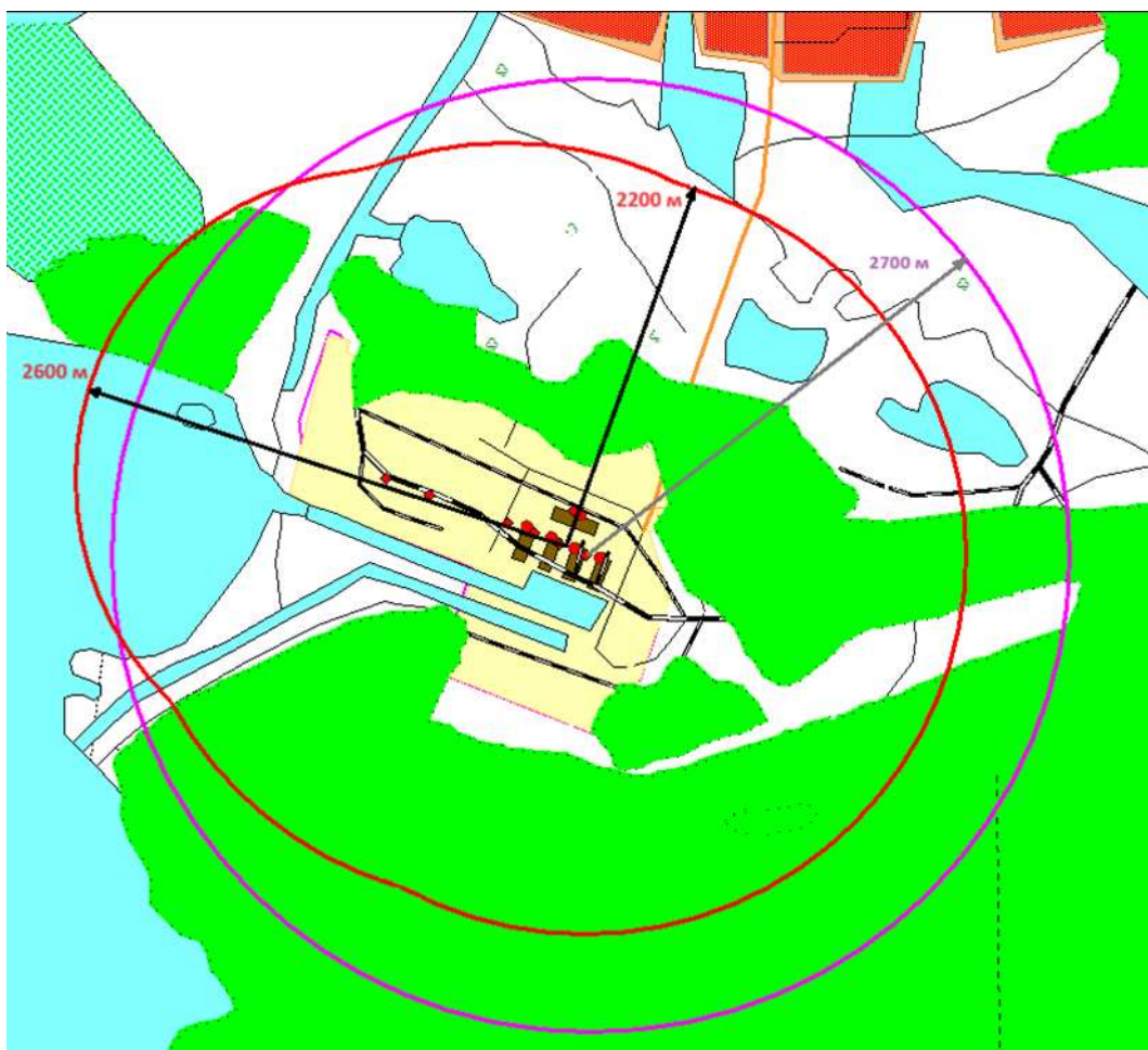
Figure 5.15 – The KhNPP SPZ boundaries are defined as a result of calculations based on the requirements of the SOU NNEGC 023:2014 [55] (in red). The existing KhNPP SPZ boundaries are shown in a purple circle with a radius of 2700 m.
